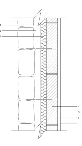
\* wall ties: recommended spacing 900mm horizontal, 450mm vertical (see BS 5628), type determined in accordance with BS 1243 and BS 8298
